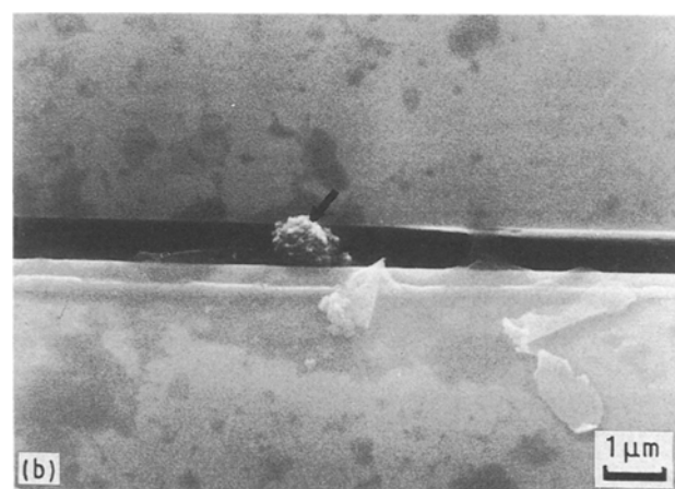
Figure 8 (a) Gap image and (b) cross-section of region C for bonded wafer pair after stabilizing at room temperature for 30 s followed by annealing at 1100\text{ }^\circ\text{C} for 10 h in \text{N}_2 .
